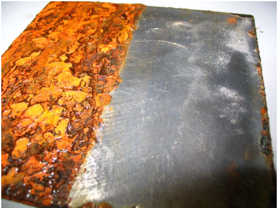
432 hours exposure: Heavy rusting and pitting on untreated side, same panel, closer look
