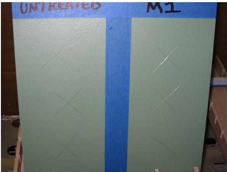
Prepped right side with M1, then primed the surface, and scoured the surface
