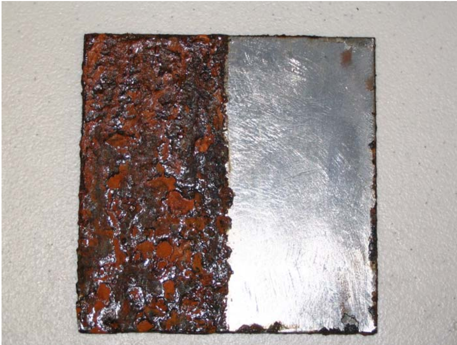
432 hours exposure: Heavy rusting and pitting on untreated side
