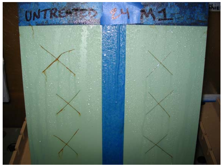
24 hours exposure: Slight rusting on untreated side
