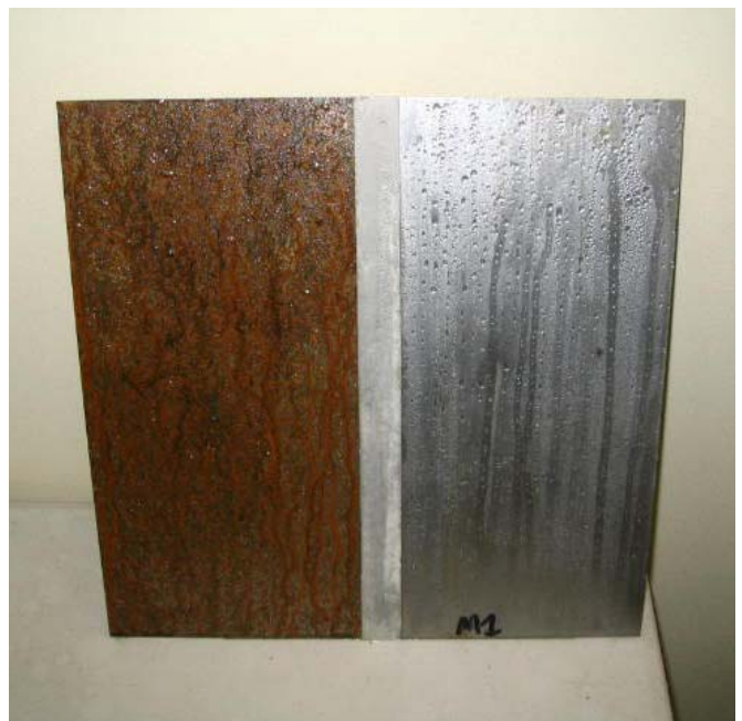
Second panel after 3 hours in QFOG
