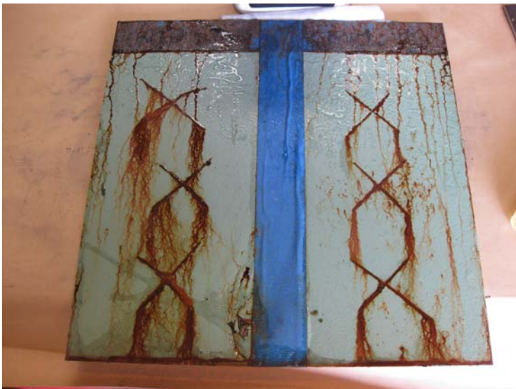
191 hours exposure: Heavy rusting and pitting on untreated side, M1 has moderate rust
